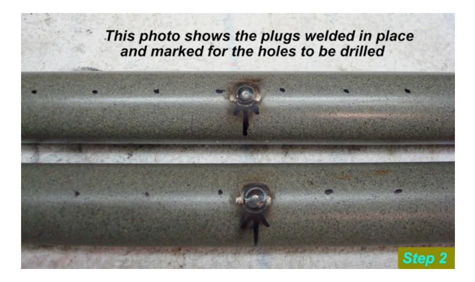
The pipe after it has been drilled. Drill 12 holes on each side of the plug. Here you can get creative as far as pattern, I drilled 3/8" holes at 1 1/2" apart offsetting the holes. If you only drill 12 holes do not drill smaller then 3/8" holes
