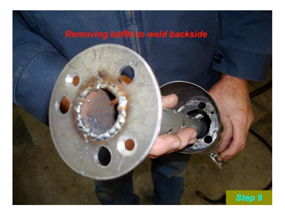
Backside welded. Now it's just a matter of grinding all your welds, making it pretty and paint with high temp paint. If your not doing the bolt in method at this point you can reinsert the baffle and weld in place. After welded in you can seal the outer edge w/ JB Weld then paint
