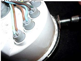
Use a dremel cutoff wheel to remove the bezel ring – cut all the way around – "Except" for enough to leave a tab for re-installation – this metal is very thin....
