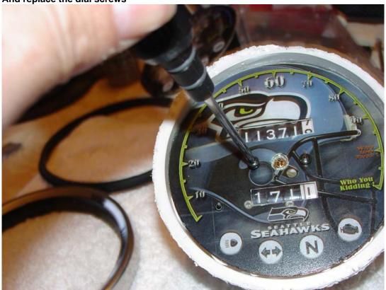
Replace your speedo needle – in the approximately the exact position you removed it from...(as close as you can get).... If you don't the speedo will not read correctly
