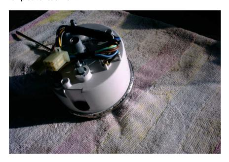
step 5.... at this point there should be enough play in the rim to enable you to gently pry the housing free from the rim, taking care not to cause any flex in the glass.
