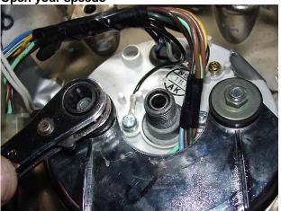
Remove the speedometer from it's housing
