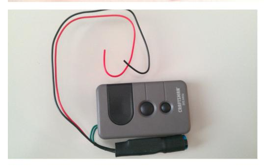
I then removed the front off of the head light dome and unplugged the headlight giving me a little more room to work. I used two crimp-on splicers to connect the remote to the head light. There are two Yellow wires running parallel to each other that power the bright beam. I connected the Red wire to one of them. I then connected the black wire to one of the black ground wires also running to the headlight connector.
