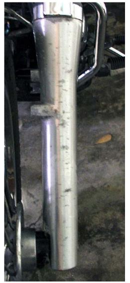
Ok I thought long and hard about how to repair the pitted and corroded lower forks on my bike, I even posted a few threads in the forum but nothing helped. So I decided to take matters into my own hands. The supplies you will need are one can of aircraft paint remover (I found it at Walmart it is in a blue can along with all the paint stripper), you will need several sheets of sanding paper in 220 320 400 600 and 1500 grit I used 2000 but I think 1500 would be good enough
