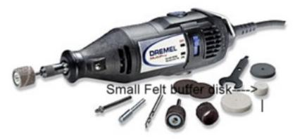
Wipe on some of the red compound with a cloth in a small area and work it in with the Dremel, on low speed. The red compound will turn black, and you will go through a number of the small felt wheels. Repeat this step a couple of times. You will not get all of the compound off with the wheel, so use a rag to work it as well. You should have a pretty good shine at this point.
