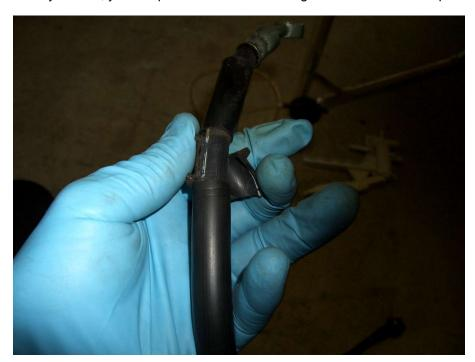
16. The Goodridge line has nice chrome fittings, and it comes with the necessary copper washers. Note that you'll need two washers on both top and bottom.
