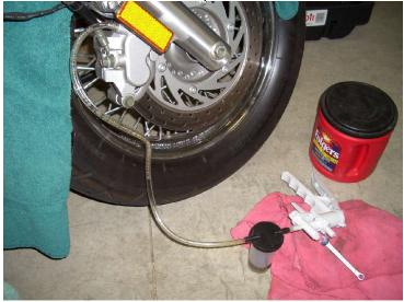
8. Pump the MityVac a few times to create vacuum, then open the bleeder valve again. Fluid will start to flow.
