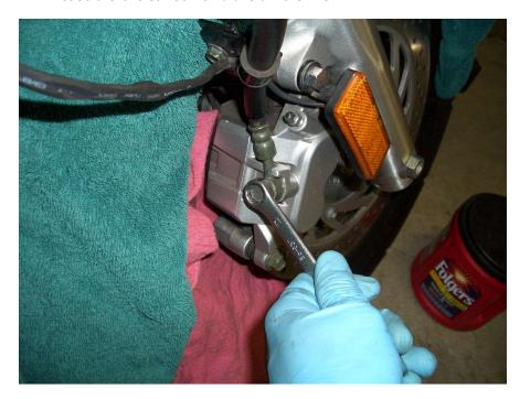
12. Now peel back the rubber boot at the top end of the line and remove it in the same way. (I put a couple of rags over the throttle cables after I took the next picture to catch the few drops of fluid that dripped out of the reservoir.)
