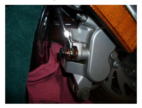
17. Route the brakeline up through the clips, reusing the thick gaskets if necessary. Attach the top end of the brake line in the same way as the bottom, using the two copper washers.
