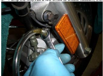
9. Surround the brake fluid reservoir with rags and open it. You should see the level of fluid fall until there is none left. Keep pumping the MityVac as necessary. Should take no more than 5 minutes to get most of the old fluid out.
