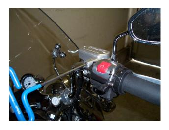
3. Tie down your front fork so that it cannot suddenly turn and spill brake fluid out of the reservoir when you have it open.
