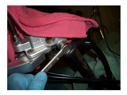
13. Now remove the old line from the clips holding it to the bike. You can just pull it straight up out of the lower clip next to the caliper.
