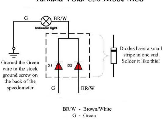
After you solder the diodes and the wires I would strongly recommend using shrink tubing on the soldered portions. Just remember to slide the shrink tubing on the wire before you solder it, otherwise you won't be able to get it on!
