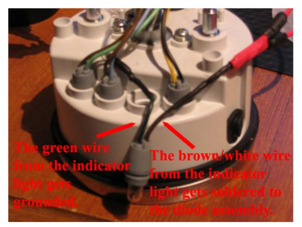
The last thing you have to do to the back of the speedometer is solder the end of the diode assembly that has two wires sticking out to the green and brown/white wires coming out of the wiring harness. One wire from the diode assembly gets soldered to the green wire and the other gets soldered to the brown/white wire. It doesn't matter which one is which.
