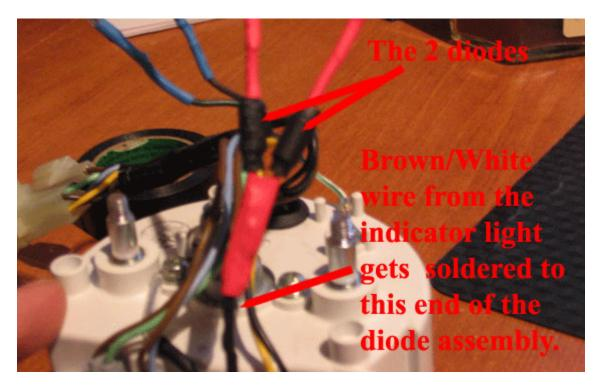
The black things are the diodes, the red is just shrink tubing around the soldered joints.
