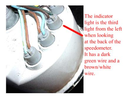
Next you will need to cut the green wire and ground the bulb to the ground screw located on the back of the speedometer face as seen below. Also reference the schematic on page one to familiarize yourself with how the wires should be cut.
