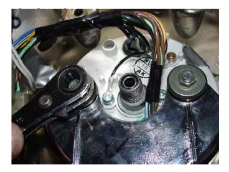
The trip meter knob is attached with a #2 metric Phillips screw down the center of the knob.
