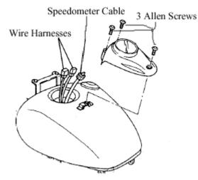
Next you have to remove the speedometer from the housing do this by removing the two nuts from the back of the housing, as seen below.
