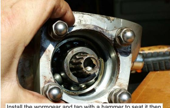
Install the wormgear and tap with a hammer to seat it then install the retainer. Remember the treads are left handed. Just tap it in thight.
