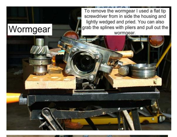
This is where I pried with a screwdriver to get the wormgear loose then used pliers to pull it out by the splines.
