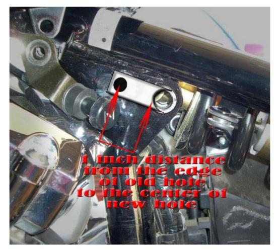
•With a center punch mark the center of the new hole, this will allow you to start drilling here and keep the bit from moving out of position.
