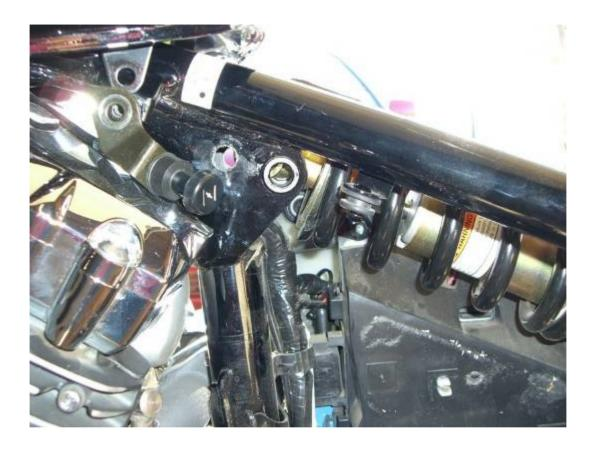
Drill with a smaller size bit and then move to ½ inch one to make a hole a half inch in diameter-<u>(take care while drilling make sure you don't drill into the wire bundle</u>).
